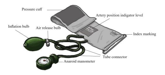
Figure 8.8: Different parts of Anaroid Sphygmomanometer
