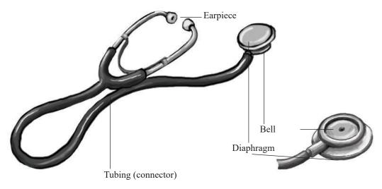
Figure 8.9: Different parts of Stethoscope
