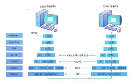
Image 5.1: Data flowing through the seven layers of OSI
